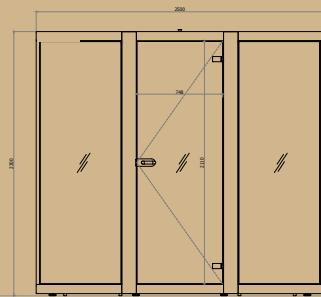
Recommended minimum ceiling height for installation 2500mm (contact us to discuss if the ceiling is lower than 2.5m).
