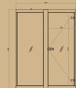
Recommended minimum ceiling height for installation 2500mm (contact us to discuss if the ceiling is lower than 2.5m).
