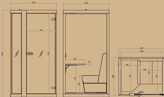
Recommended minimum ceiling height for installation 2500mm (contact us to discuss if the ceiling is lower than 2.5m).
