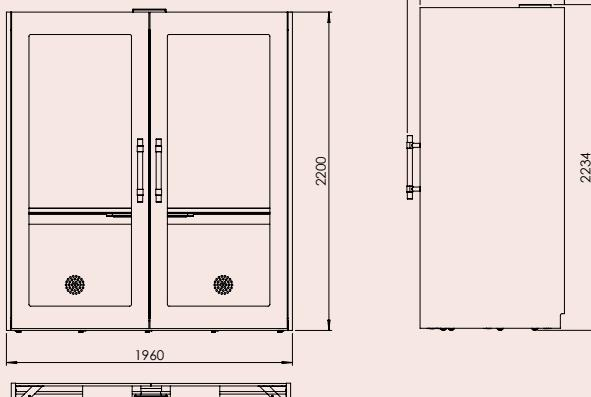
Recommended minimum ceiling height for installation 2500mm (contact us to discuss if the ceiling is lower than 2.5m).
