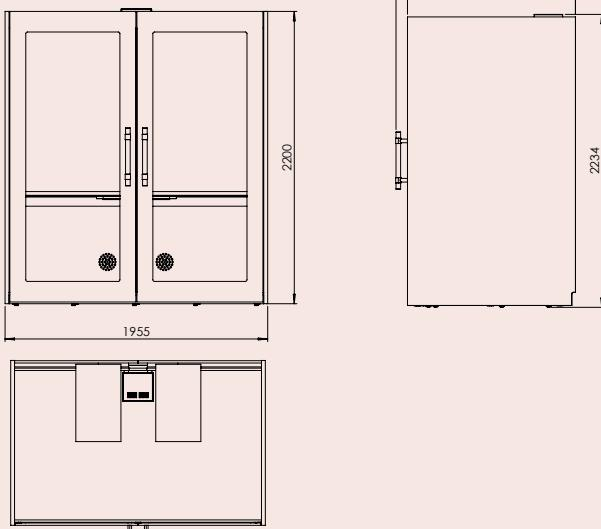
Recommended minimum ceiling height for installation 2500mm (contact us to discuss if the ceiling is lower than 2.5m).
