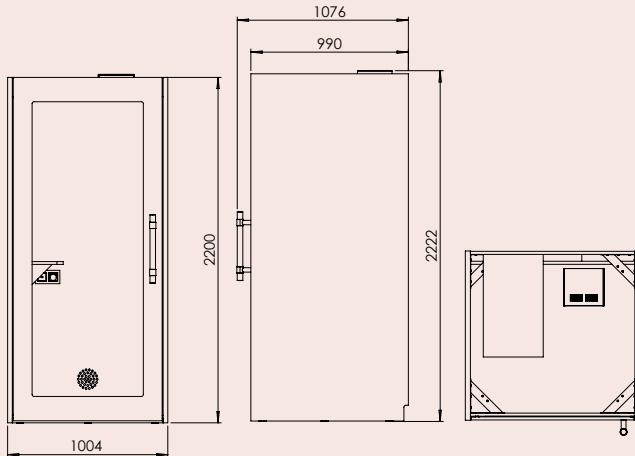
Recommended minimum ceiling height for installation 2500mm (contact us to discuss if the ceiling is lower than 2.5m).
