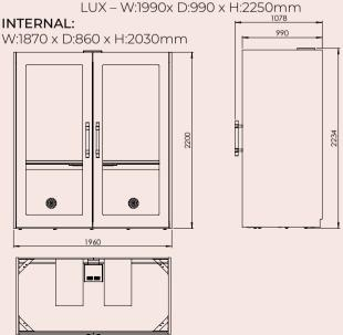
Recommended minimum ceiling height for installation 2500mm (contact us to discuss if the ceiling is lower than 2.5m).
